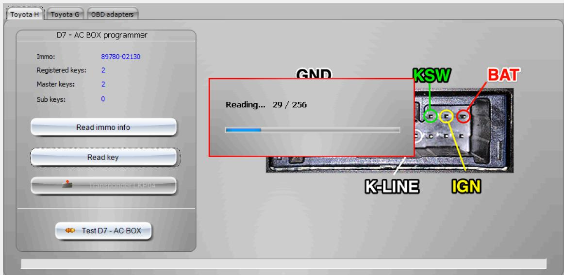
8) After reading, prepare the LKP04 transponder and press write.
